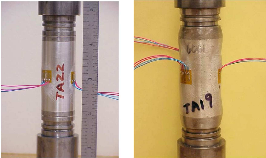
Figure 5.1. Strain gaged aluminum specimens
