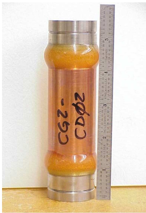
Figure 5.3. Right circular cylinder of Castlegate sandstone jacketed in copper with end caps attached.
