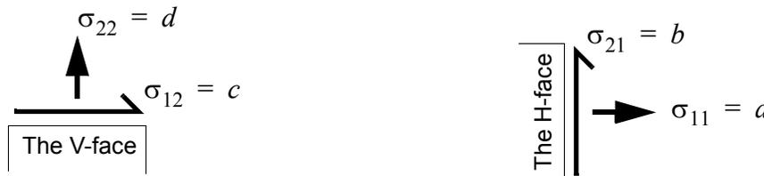
Figure 3.1. The H and V faces of the "stress" element. The outward normal of the H face is horizontal and the outward normal of the V face is vertical.
