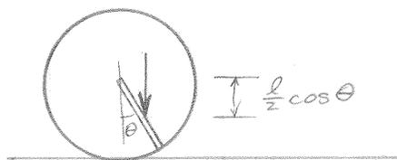
This problem is perfect for energy methods because the only position for which the rod's moment of inertia about the IC is known exactly is when the rod is vertical down, which is the pos'n of max K.E.
