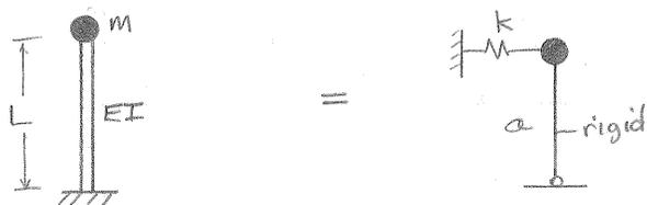
Find  $k$  &  $a$  for the two systems to be dynamically equivalent with respect to the translation and rotation of the mass  $m$ .
