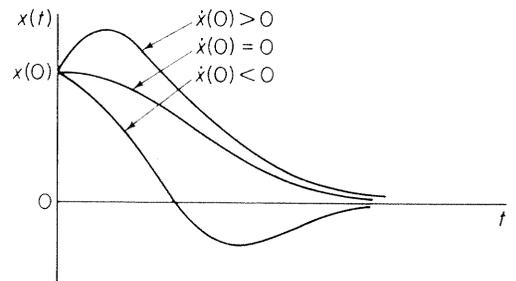
Figure 2.3-5. Critically damped motion  $\zeta = 1.0$ .
