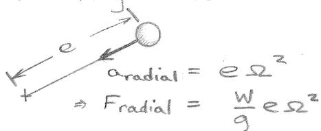
$\Rightarrow$  Force on block due to two rotating imbalances is
