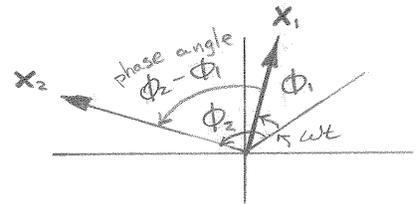
$$\begin{aligned} A_1 \cos \omega t + A_2 \sin \omega t &= A \cos(\omega t - \phi) \\ \text{or } A_1 \angle 0 + A_2 \angle -\pi/2 &= A \angle -\phi \quad \text{where:} \end{aligned} \quad \left. \begin{aligned} A_1 &= A \cos \phi \\ A_2 &= A \sin \phi \end{aligned} \right\} \text{CBS}$$
