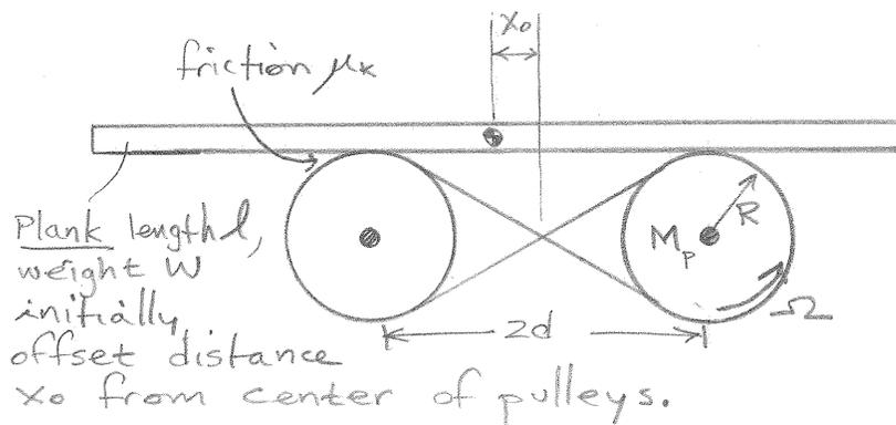
REQ'D How long will it take for the system to come to a rest assuming  $\Omega$  is initially large?
