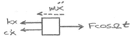
$$m\ddot{x} + c\dot{x} + kx = F\cos\Omega t \quad \text{or} \quad \ddot{x} + 2\zeta\omega_n\dot{x} + \omega_n^2x = \frac{F}{m}\cos\Omega t \quad (1)$$
