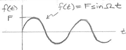
$$x = \frac{F/\sqrt{km}}{\omega_n^2 - \Omega^2} (\omega_n \sin \Omega t - \Omega \sin \omega_n t)$$
